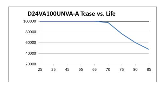
The Data curve provided predicts the LED Driver life based on the case temperature measured at the Tc location identified on the label or specification sheet. The Telecordia SR-332 standard is used to generate the prediction curves.
