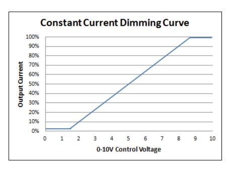
Dimming output is Analog for use in Constant Current Mode
