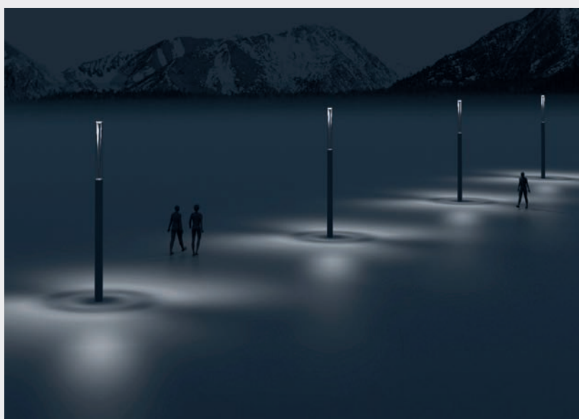
Simulation Rush 750311 38W 3000K Optics 360° Luminaires interdistance 12mt.
