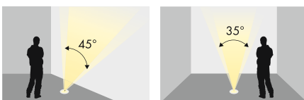
Asymmetrische Linse 45°/35° / Asymmetrical lens 45°/35°
