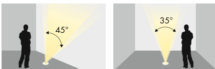
Asymmetrische Linse 45°/35° / Asymmetrical lens 45°/35°
