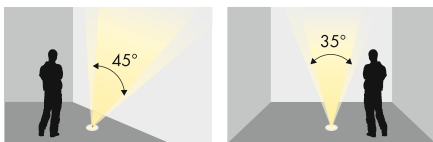
Asymmetrische Linse 45°/35° / Asymmetrical lens 45°/35°
