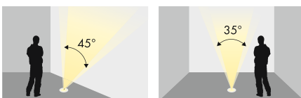
Asymmetrische Linse 45°/35° / Asymmetrical lens 45°/35°
