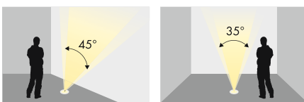
Asymmetrische Linse 45°/35° / Asymmetrical lens 45°/35°
