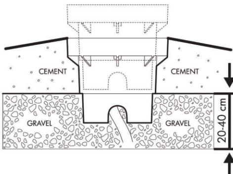
**UK** To ensure good drainage and to avoid water stagnation, provide a 30 cm draining gravel layer or a draining pipe system. **Caution! Do not install the luminaire on hollow areas or on water stagnation areas** (Fig. 1).
