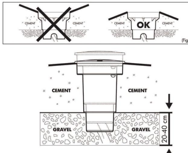
**UK** To ensure good drainage and to avoid water stagnation, provide a 30 cm draining gravel layer or a draining pipe system. **Caution! Do not install the luminaire on hollow areas or on water stagnation areas** (Fig. 1).
