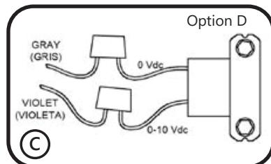
Connections for wired external dimming.
