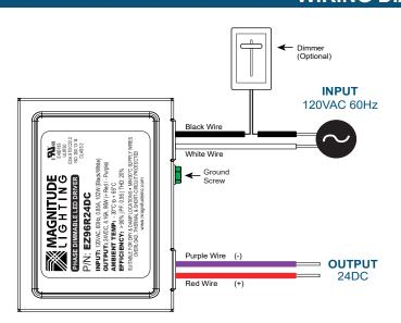
Do not install PWM low voltage controllers on the output without consulting with Magnitude Lighting.
