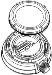
Figure 1 – Lens installation
