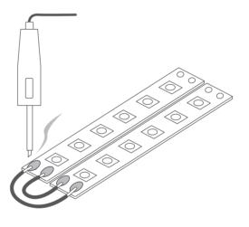
**OPTIONALLY:** The LED strips can also be connected using a system of LED strip connectors. More information at <a href="https://www.klusdesign.com">www.klusdesign.com</a>
