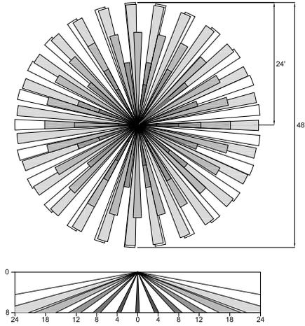
Sensor Lens Coverage and Detection Patterns
