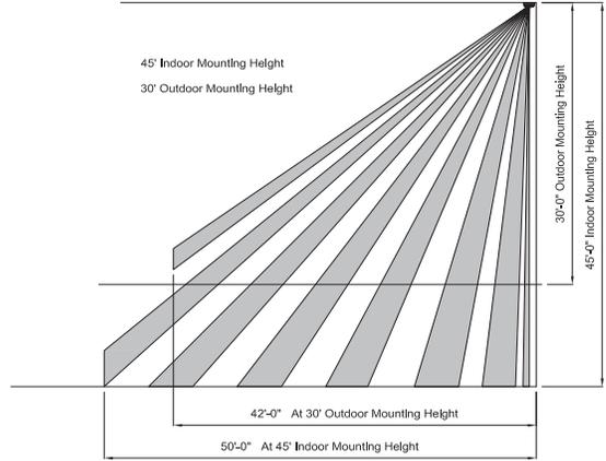
Sensor Lens Coverage and Detection Patterns
